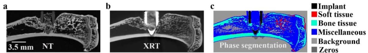
Figure 1. Representative sagittal slices of registered NT image (a), XRT image (b), and phase segmentation obtained from the registration of the images (c). Both NT and XRT images are displayed in the grey scale interval 0-255.
